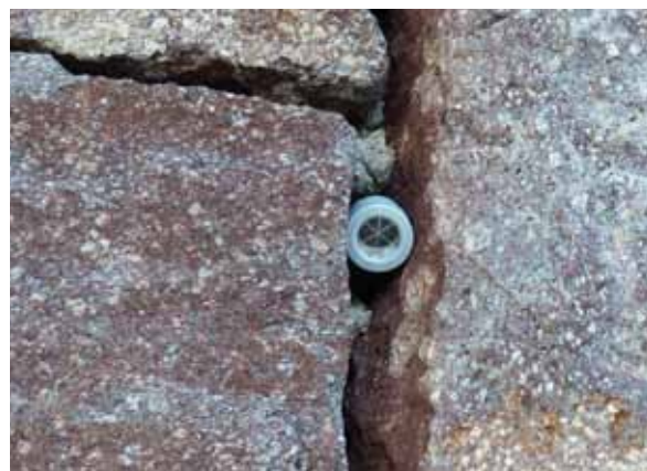
RSMP10 placeable in the smallest column
