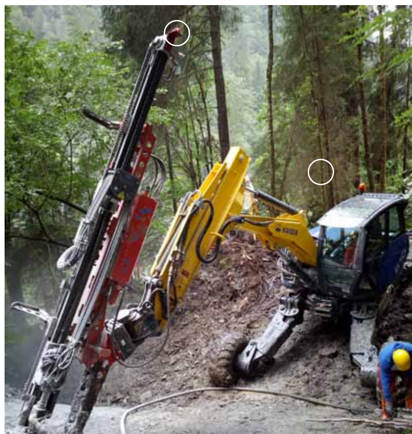
Example of the use of RS193rM as a fixed point on different surfaces and for the exact alignment of the drill carriage.
